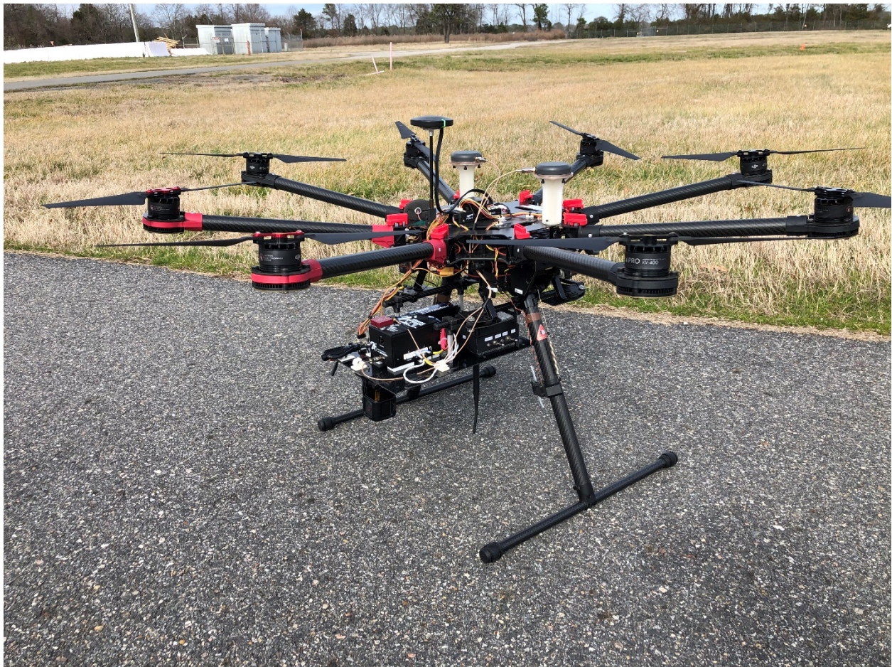
Figure 3 - Flight test vehicle configured with Safeguard as an IFTS.
